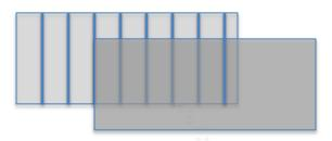
The two layers of film have fiber threads in between to reinforce the structure of the film.
