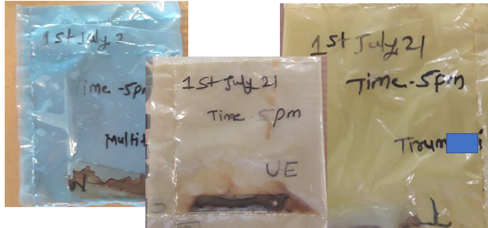
Fake VCI failed in 24 hours
